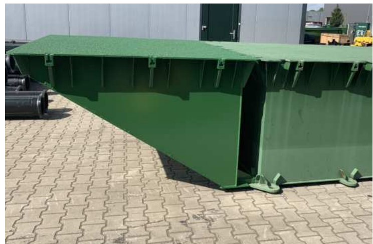
Bowpiece to connect the platform to land
